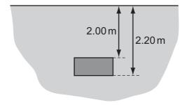
What is the difference in pressure between the top and bottom surfaces of the block?
